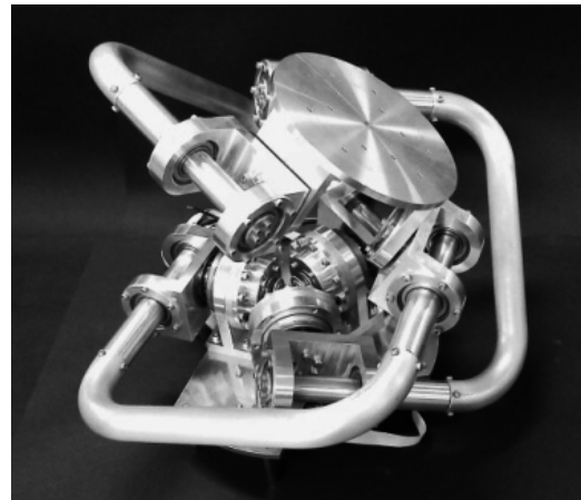
Fig. 1 A Zero-DOF 3-UU parallel mechanism (2)
