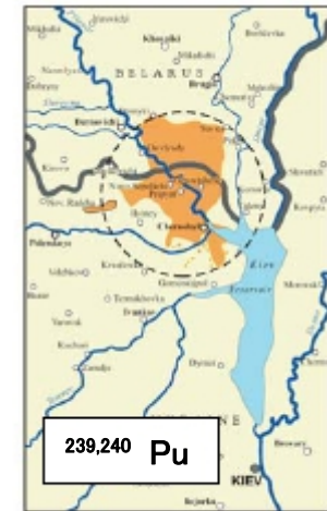
FIG. 3.9 Areas (orange) where the surface ground deposition of 239,240 Pu exceeds 3.7 kBq m⁻² [54].
