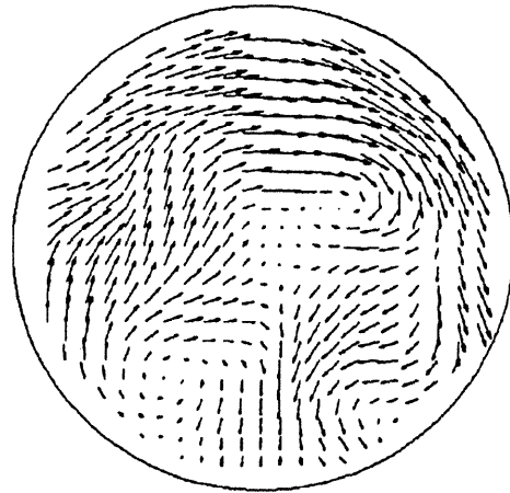
Fig 5a: Velocities in combustion chamber at 11.5° atdc with swirl ratio of 4.0
