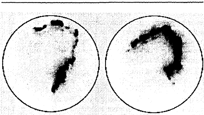
Figure 6 LII soot images from two different engine cycles. Image location is 1.9 cm (0.75 in.) below the cylinder head, 17° ATDC.
