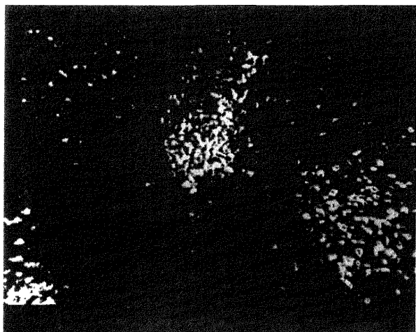
Fig.9 Polarization ratio pattern from a spray cross section at 30 mm from the nozzle in ignition conditions /4/.
