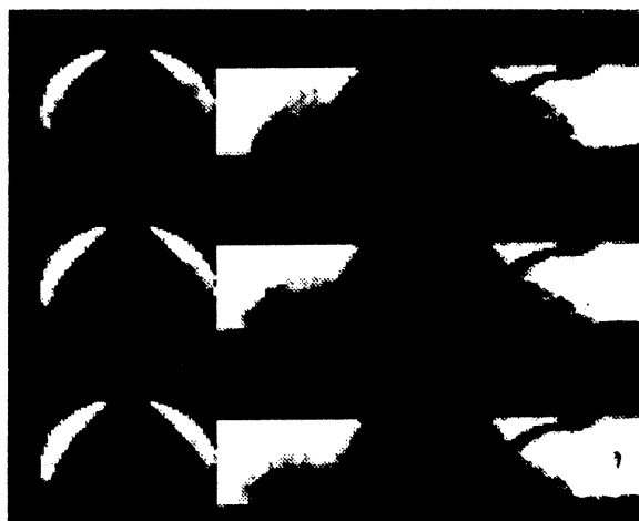
Figure 10. A sequence of orthogonal schlieren images of the fuel spray. These images were recorded at 6000 frames/sec.
