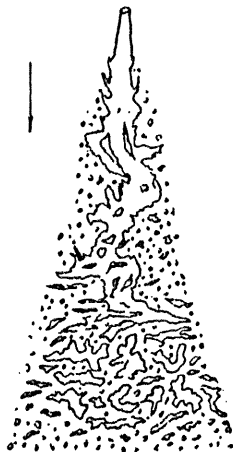
Fig.4 Break up of fuel spray ( Pa = 0.89 MPa )
