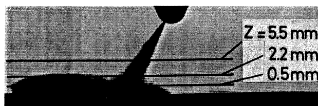
Fig.4 Shadow photograph of an impinging spray \theta=30 deg., L=13.4 mm, d_0=0.35 mm, t=0.7 ms
