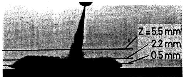
Fig.14 Shadow photograph of an impinging spray \theta=15 deg., L=20.0 mm, d_0=0.25 mm, t=1.1 ms
