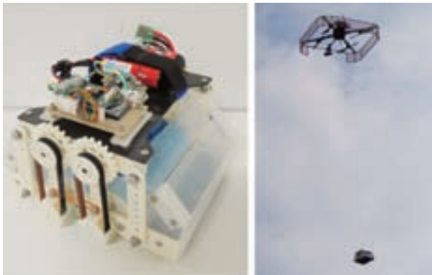
Fig.5: Soil-sampling device (left) and an overview of the system (right).
