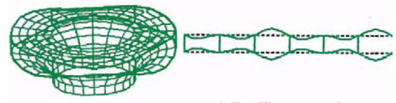
Fig.3 Example of excitation mode of pump turbine runner
